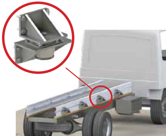
Figure 2. Anti-vibration systems mounted on the VCLM for impact mitigation
